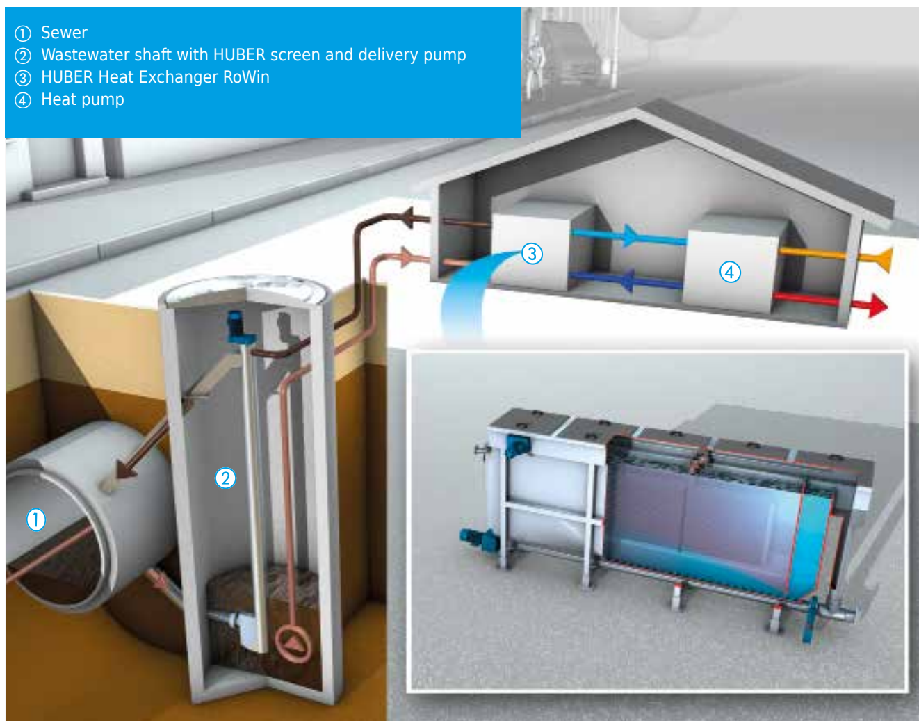
HUBER ThermWin system for the recovery of energy from wastewater.
