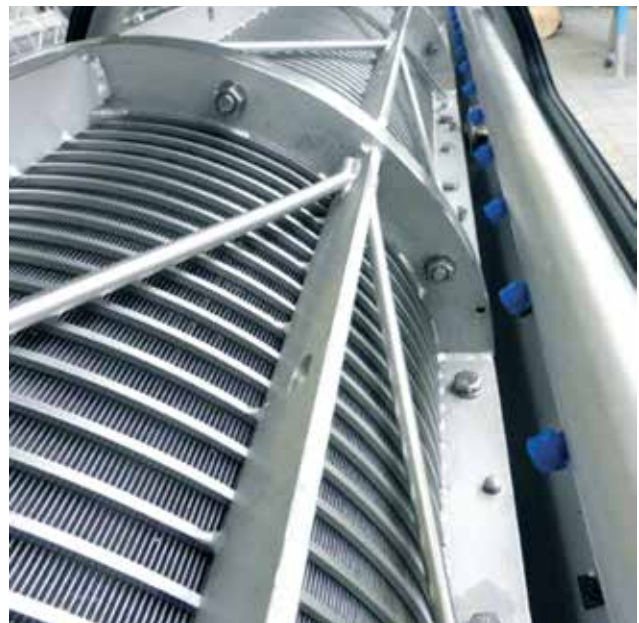
Sturdy wedge wire basket made of stainless steel.
