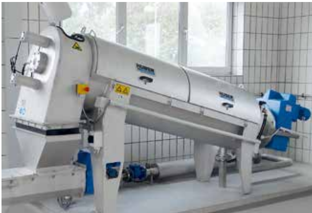
Stationary mounted Q-PRESS® 440.2 for 3 m 3 /h.
