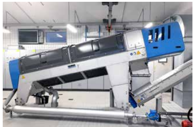
Digested sludge dewatering up to 30% DR.
