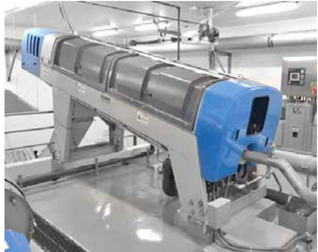
Q-PRESS® 620.2 for surplus sludge dewatering.
