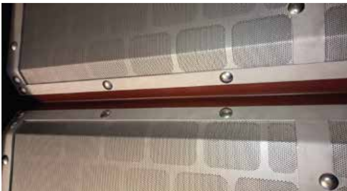
The "no pass" polyurethane sealing system ensures that no unscreened wastewater passes the screening elements.
