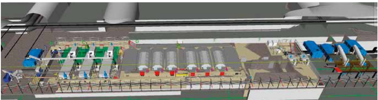
Fig. 4: River and sea outfall with 6 HUBER Drum Screen LIQUID units as replacement for a primary settling tank.
